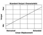
**Output Characteristic:** Plunger extended 10 mm<sup>\*</sup> from mounting face at start of normal travel. Note: where dome end option is fitted add 5 mm. The output increases as the plunger extends from the sensor body, the calibrated stroke is between 2 mm and 50 mm.
